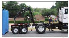
Top: The dolly is lowered into position by the tractor-mounted boom. Middle: As the near end of the container is lifted by the boom, the dolly is powered underneath by remote control. Bottom: The near end of the container has been lowered onto the tractor, everything has been secured and the M1000 is ready to roll
